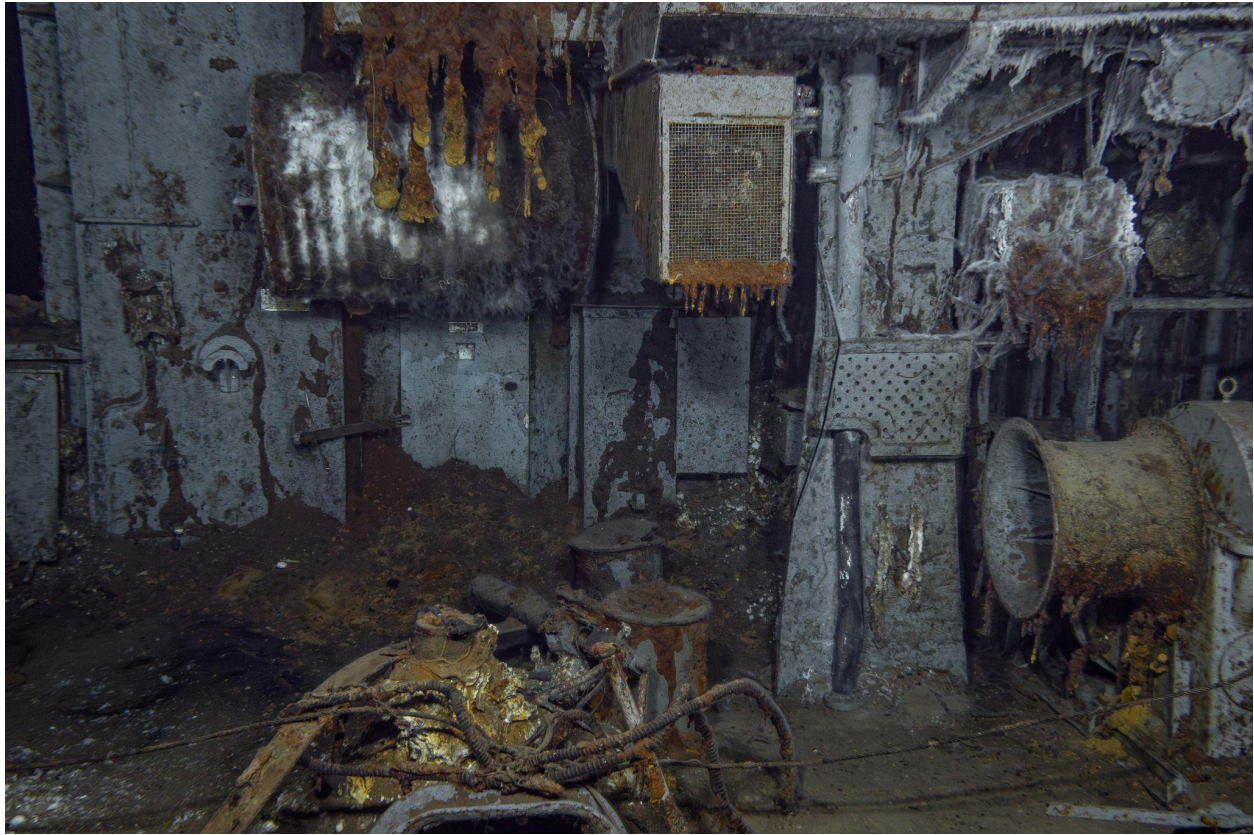
A view of machinery on the lower port aft quarter, showing a firefighting hose roll covered in an unidentified bacterial mat.
