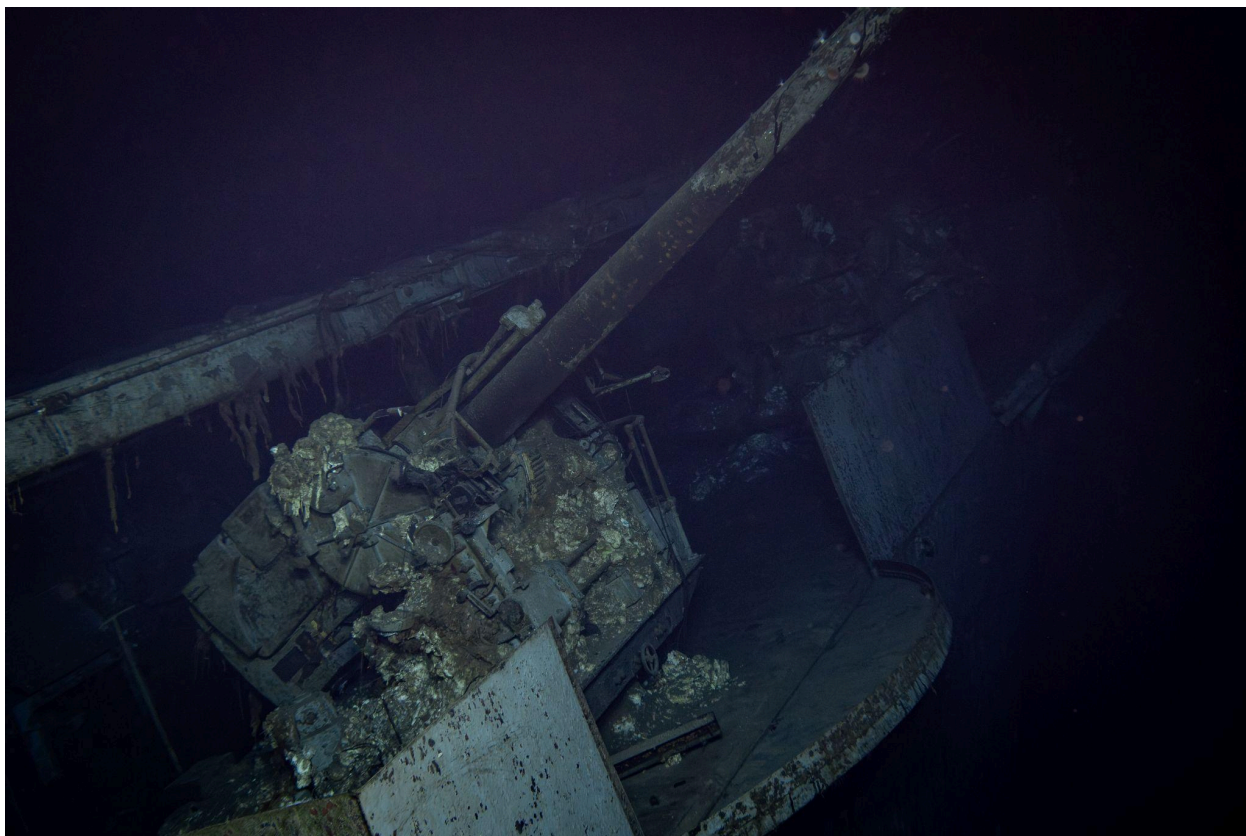
A 5-inch gun in the port aft gun gallery. The guntub shield has been removed, likely in preparation for jettisoning the gun during salvage efforts to correct Yorktown's list to starboard before being torpedoed by I-168.
