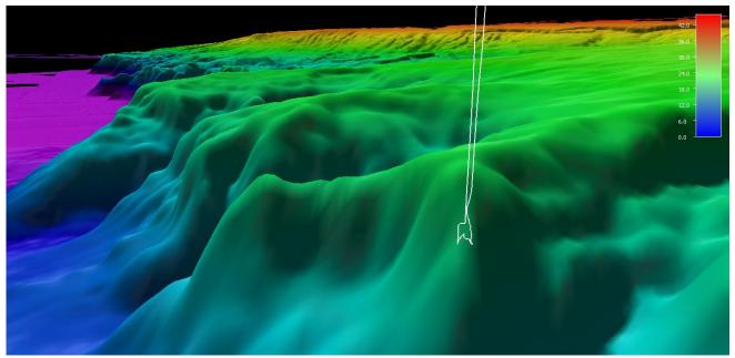
Smoothed ROV dive track in white on the bathymetry, 3x vertical exaggeration, depth in meters.
