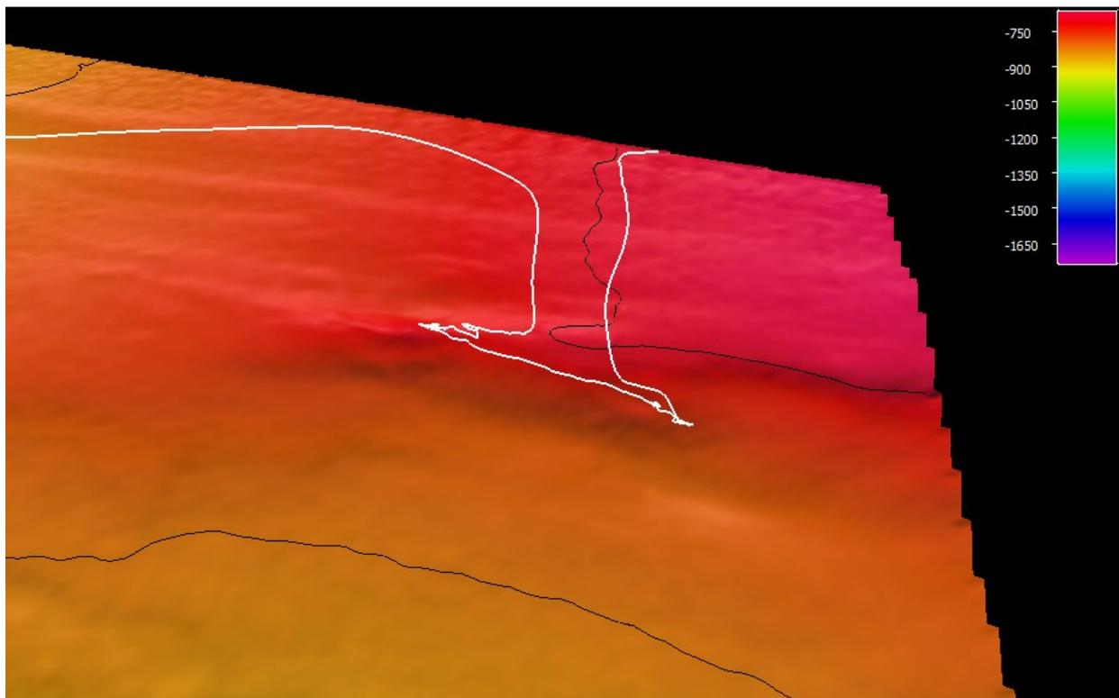
Smoothed ROV dive track in white on 25x25 cell size bathymetry, 1x vertical exaggeration, depth in meters, 10 meter contours.
