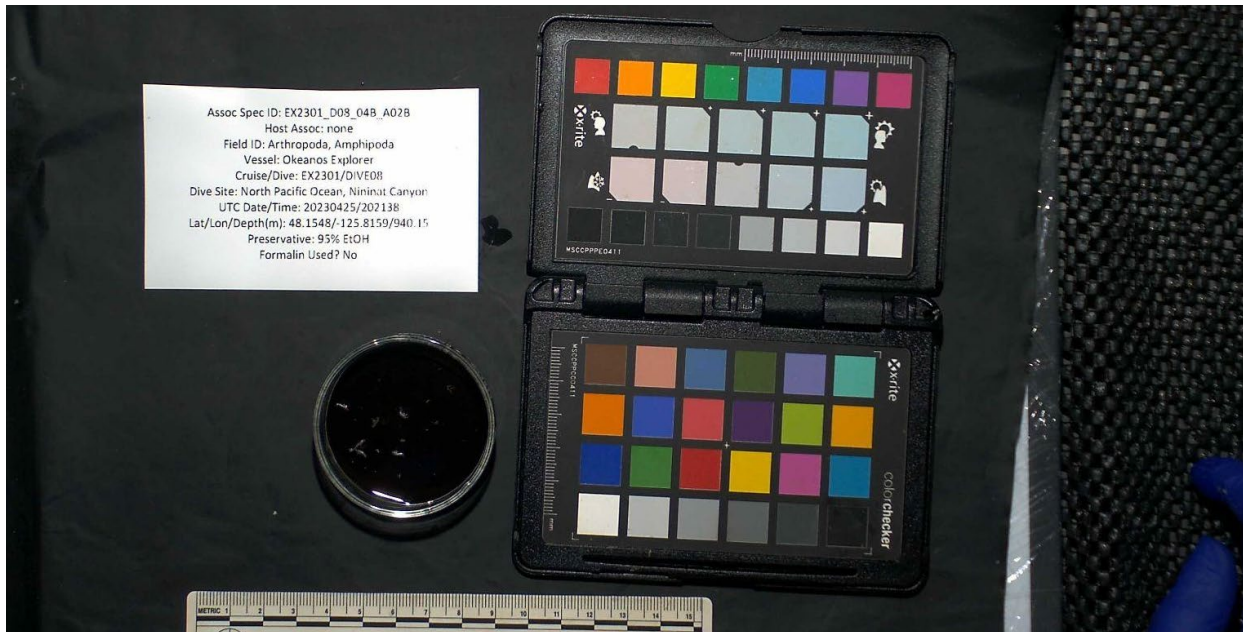
Associate amphipod samples in laboratory photo with sample label, scale bar, and color chart.
