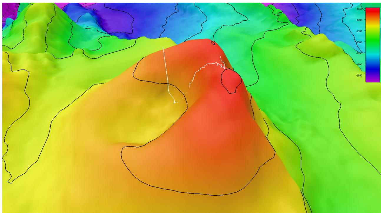
Smoothed ROV dive track in white on 25x25 cell size bathymetry, 3x vertical exaggeration, depth in meters, 10 meter contours.
