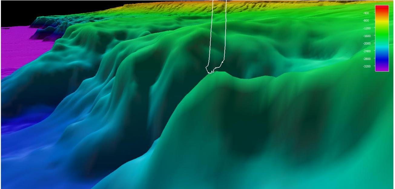
Smoothed ROV dive track in white on the bathymetry, 3x vertical exaggeration, depth in meters.
