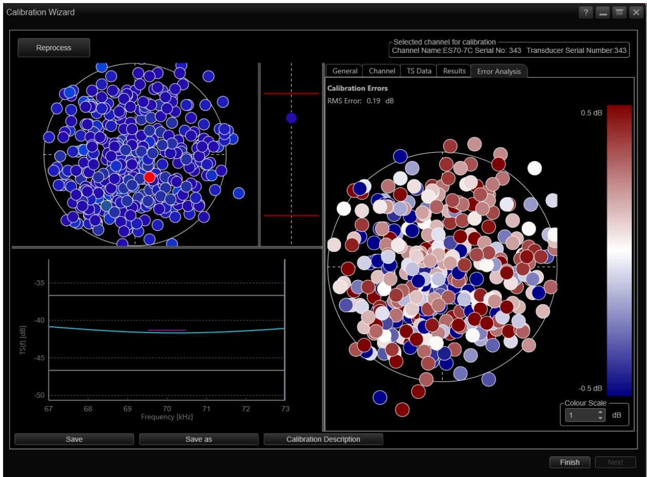
Figure 61. Screenshot of EK80 Calibration Wizard error analysis for 70 kHz calibration at 1.024 ms in continuous wave (CW) mode.
