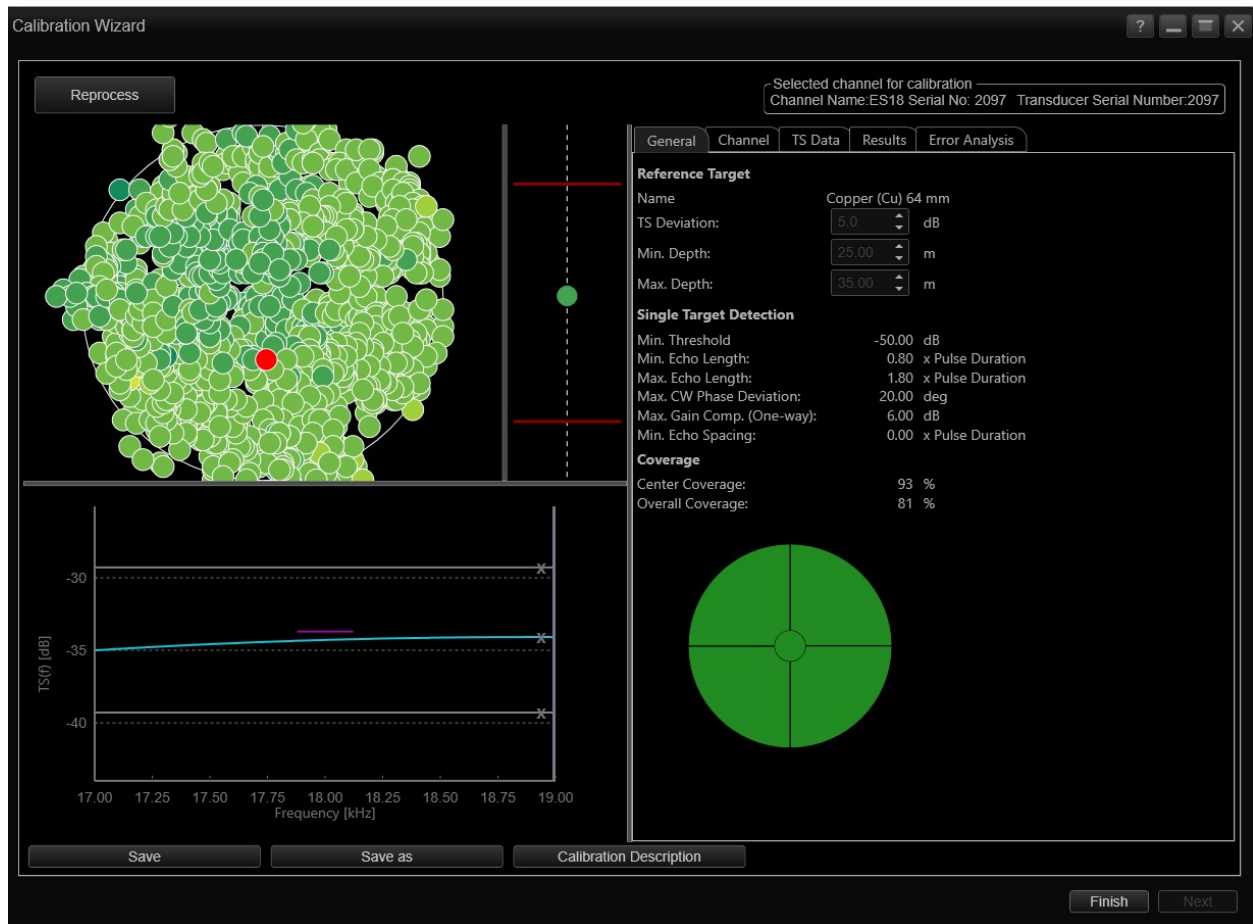
Figure 15. Screenshot of EK80 Calibration Wizard general results for 18 kHz calibration at 4.096 ms.
