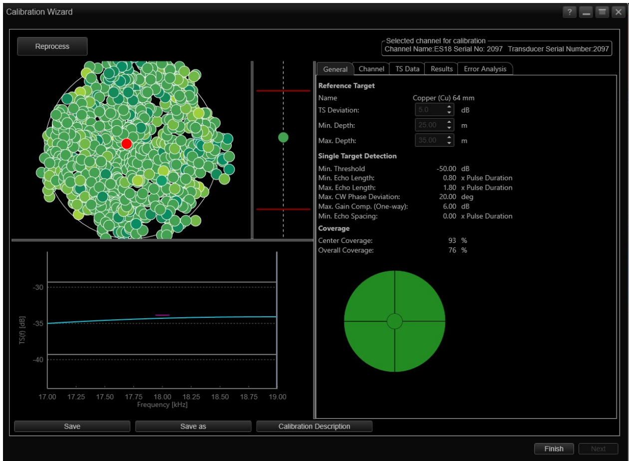
Figure 14. Screenshot of EK80 Calibration Wizard general results for 18 kHz calibration at 8.192 ms.
