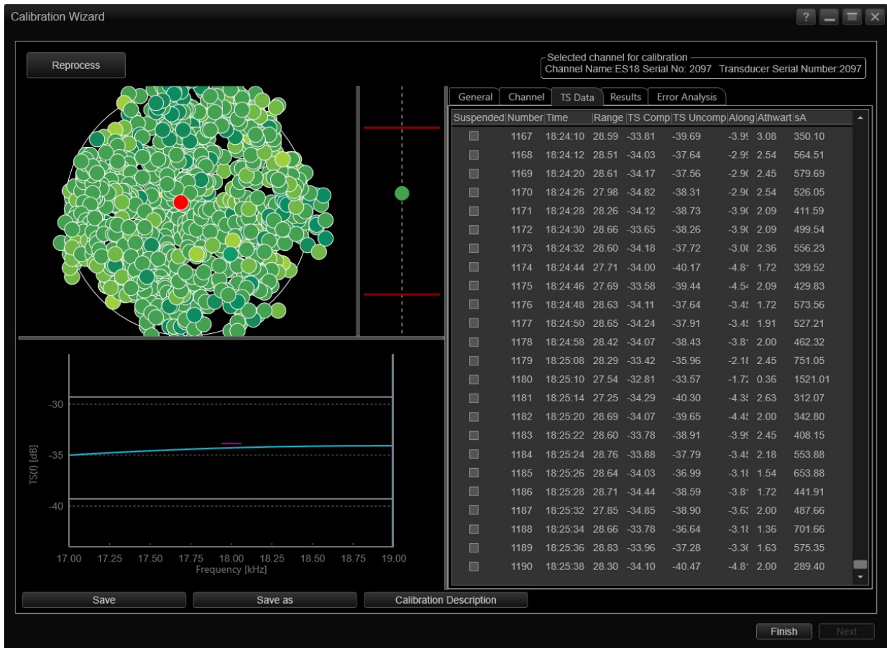
Figure 27. Screenshot of EK80 Calibration Wizard TS results for 18 kHz calibration at 8.192 ms.
