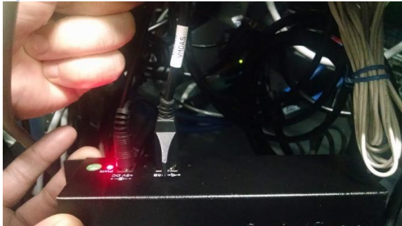
Figure 6. UHDAS cable connected to serial cable box
