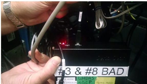
Figure 6. UHDAS cable connected to serial cable box
