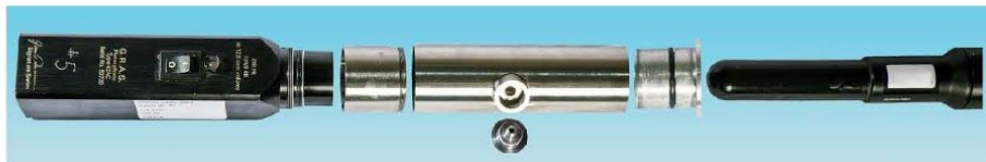
Figure 4. Split view of a G.R.A.S. 42AC pistonphone calibrator with an M36 hydrophone.
