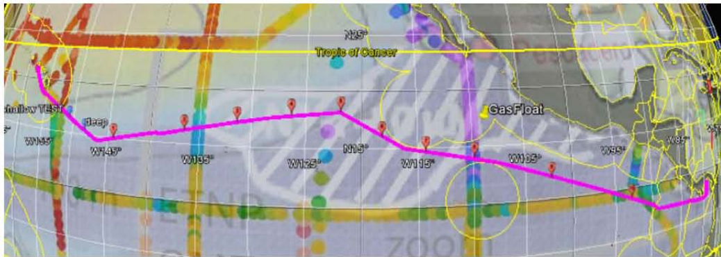
Figure 1: Map showing approximate locations of 10 CTD stations (red icons) along the cruise track. We would like to perform two test casts (blue icons) early on in the cruise, one shallow (~200 m) and one deep (600 m) to provide training to all operators and ensure proper operation of the sampling equipment.
