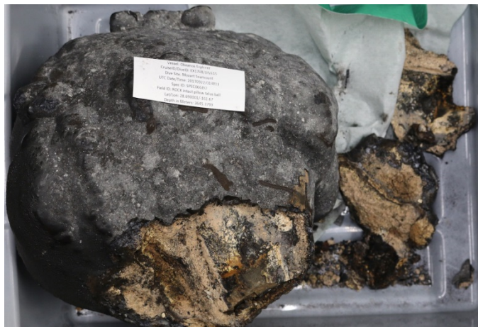
Figure 16. Laboratory photo of “pillow talus ball” (sampled on Dive 15) in Figure 15 showing interior layers of materials and polymetallic crust. Diameter of main sample is approximately 30 cm.
