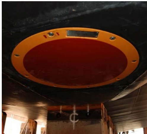
EK60 18kHz Transducer, installed May 2011. Arrows point towards the bow of the ship. The transducer is on the port side of the ship.
