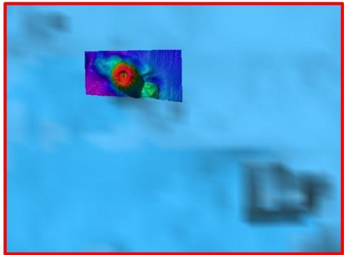
Figure 4. Showing the level of detail mapped by the EM302 multibeam, versus satellite derived bathymetry.
