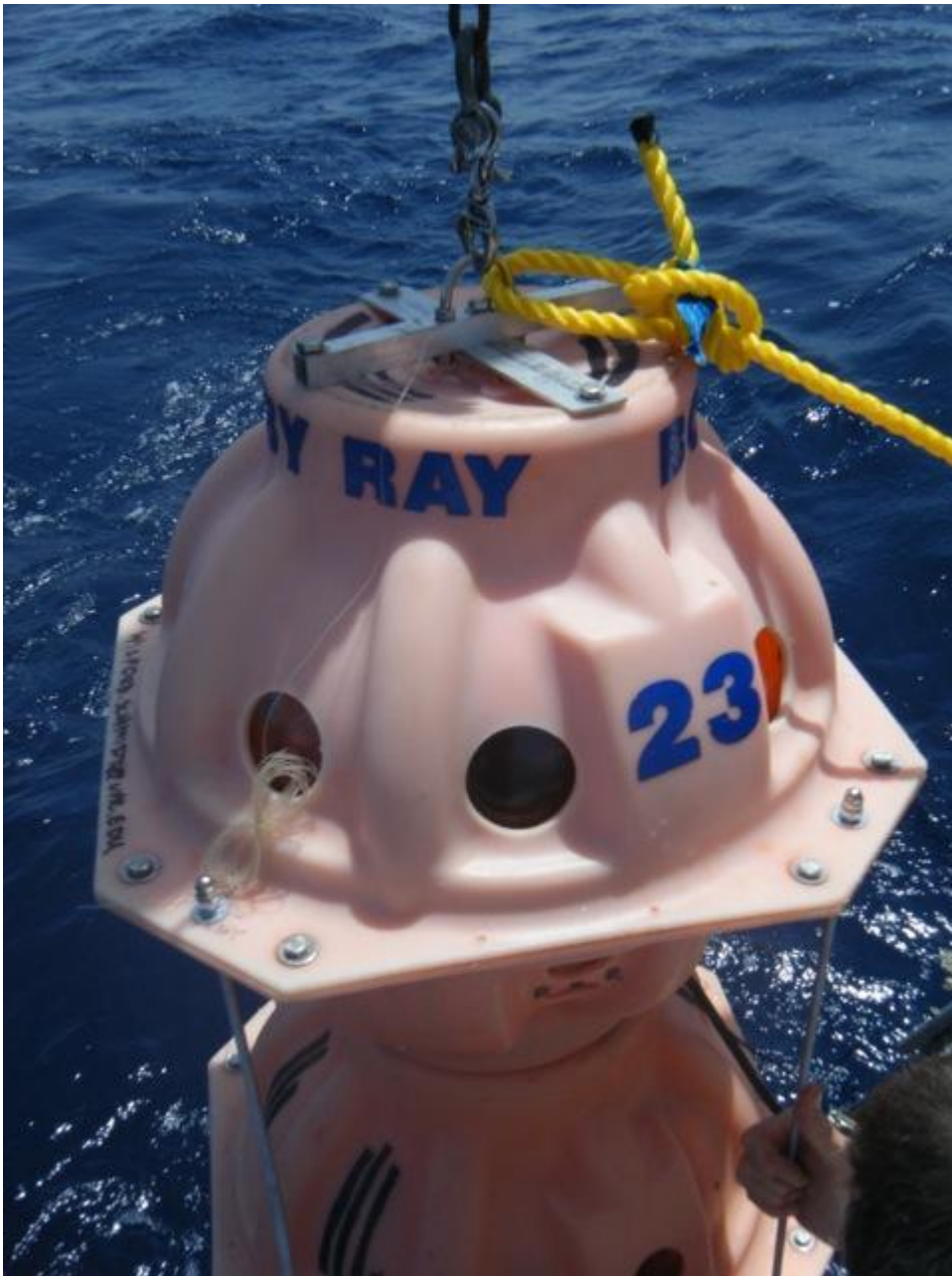
Figure 3. Close up image of free vehicle attachment mechanism.
