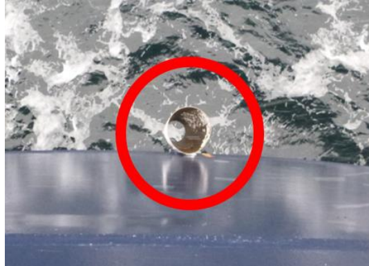
Figure 8. A line hazard with sharp edges on the forward starboard quarter
