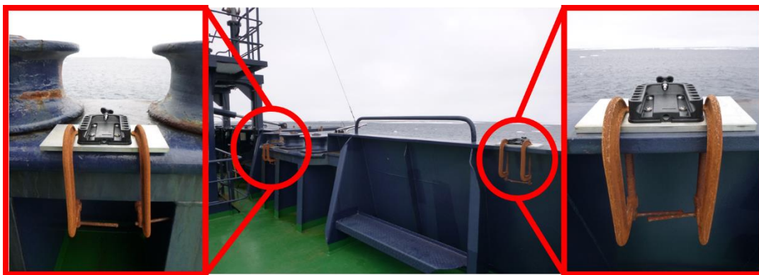
Figure 4. Detail of bow reel mounts. Mount on left is center bow mount for securing bow reel throughout deployment and calibration; mount on right is starboard bow mount for temporarily securing starboard reel during line deployment and port line movement.
