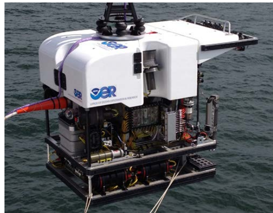
NOAA's new 6000m, two-body ROV will be used to acquire high definition visual data of unknown and poorly know areas during the 2013 Expedition.
