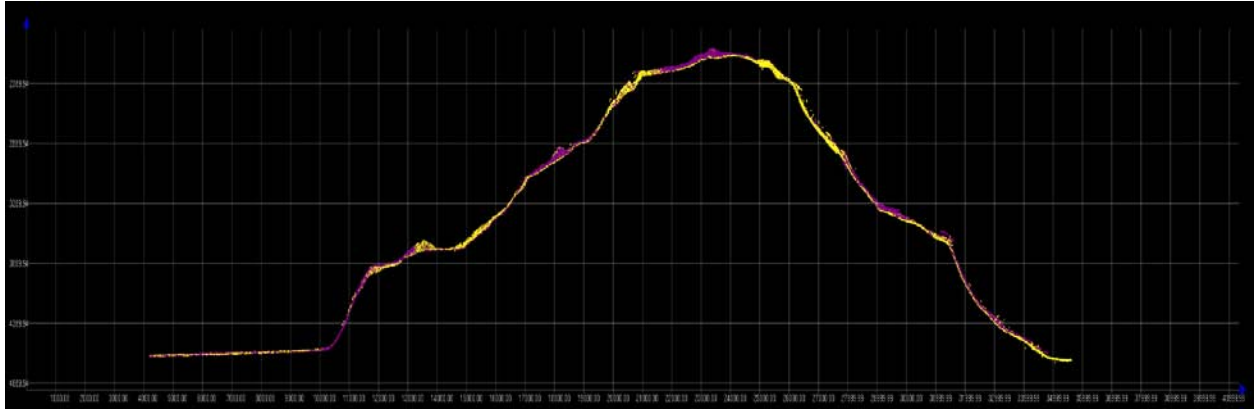
Figure 2. Screen grab of subset editor in CARIS HIPS showing agreement of cross lines (yellow) with main scheme lines (Purple). Image credit: NOAA.
