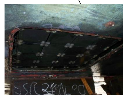
Sub-bottom Profiler Transducers Model: KEL5701-3.5kHz without Acoustic Window
